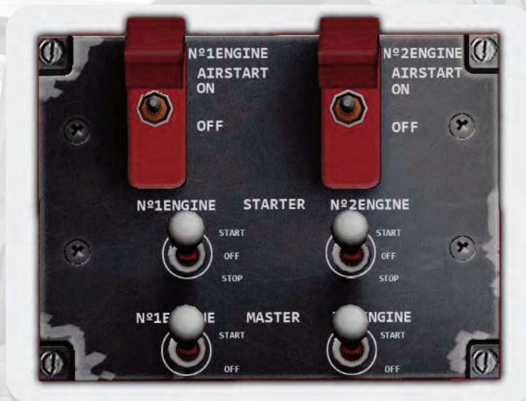
T-2B, T-2C, T-2D & T-2E Engine Control Panel
